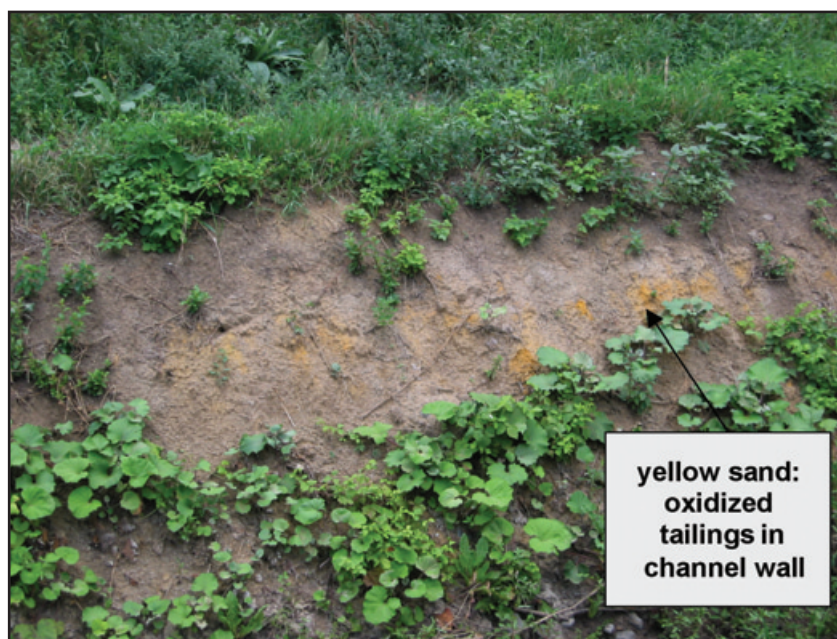
Figure 4. Oxidized heavy metal-bearing tailings deposited on the floodplains below the Gyongyosoroszi tailings dump (photo: S. Sommer).
