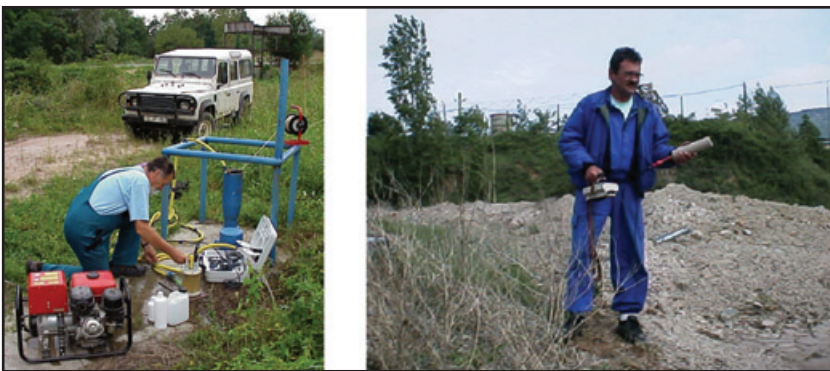
Figure 7. Monitoring system at the Mecsek Uranium Mines. Water and radiological monitoring on and around the mine site.
